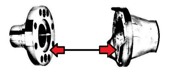
At ride height, measure between the MOUNTING SURFACES
